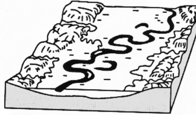
(4) Stream in old age. Wide, heavily eroded valley. Nearly flat slope. Very low velocity. Many meanders.
